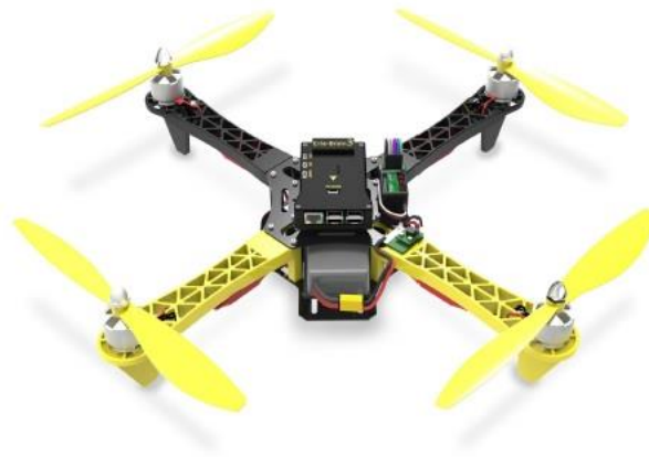
Figure 7: Original drone arms to be redesigned
